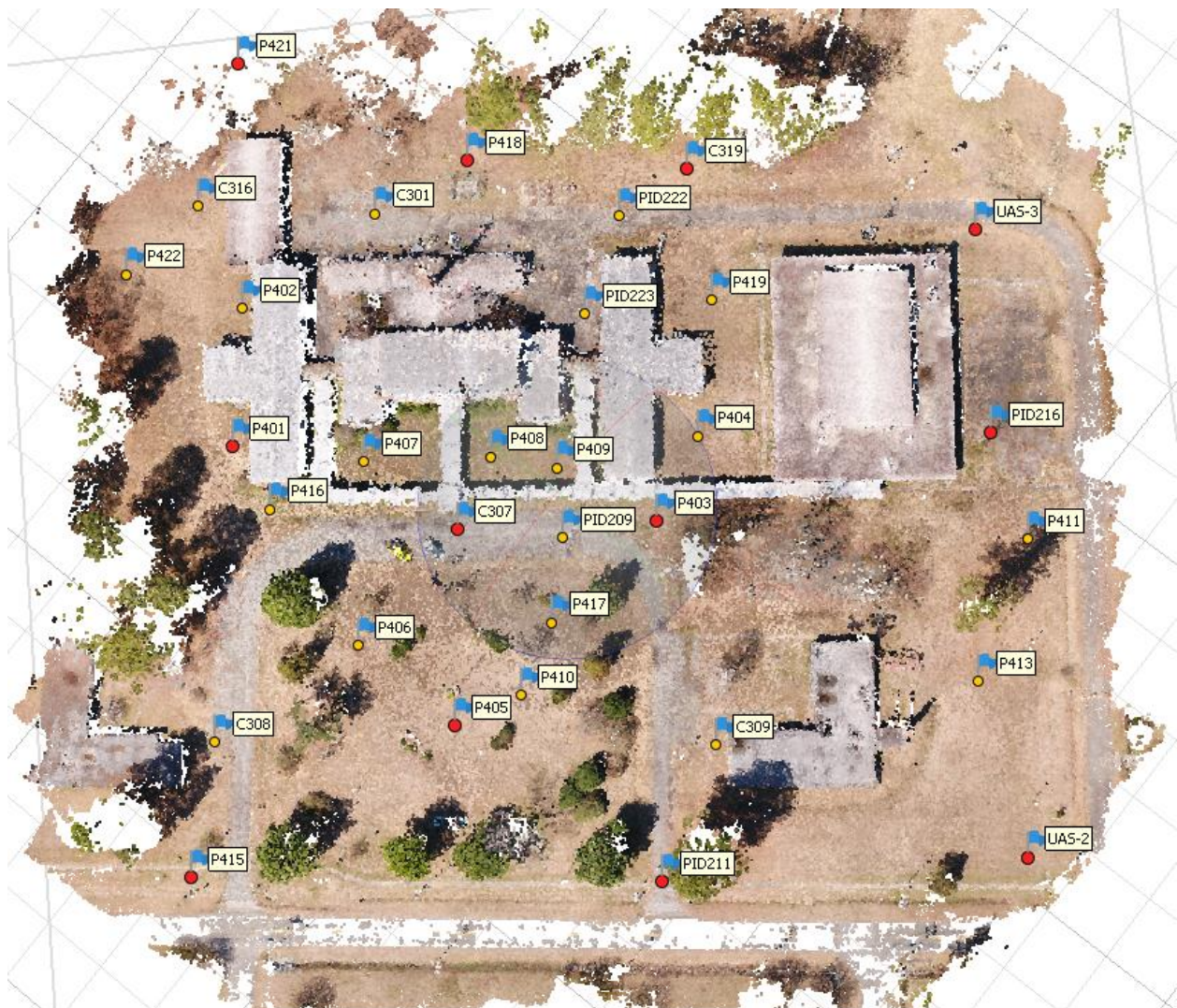
Figure 9.3 The Layout of GCPs and Checkpoints
