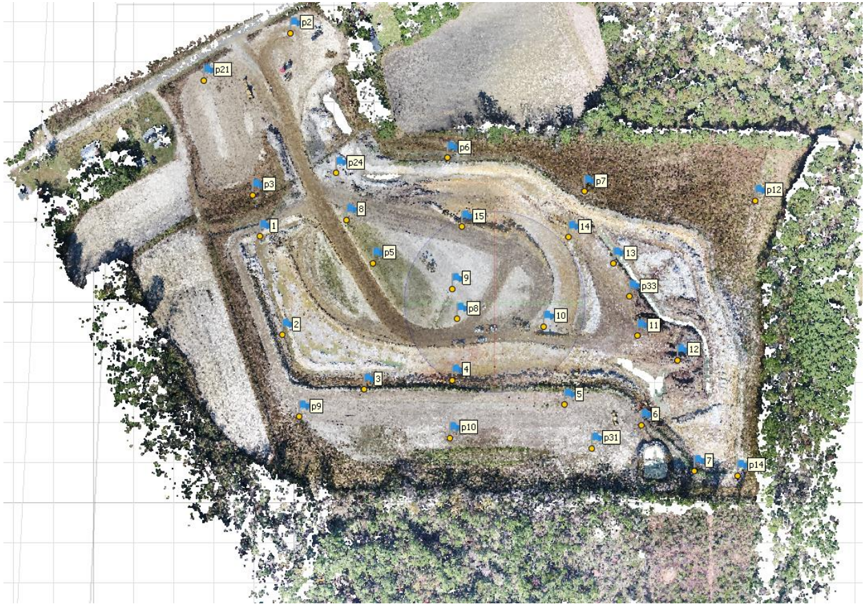
Figure 3.9 R2303-E Pit Site Aeropoints and Surveying Points Layout
