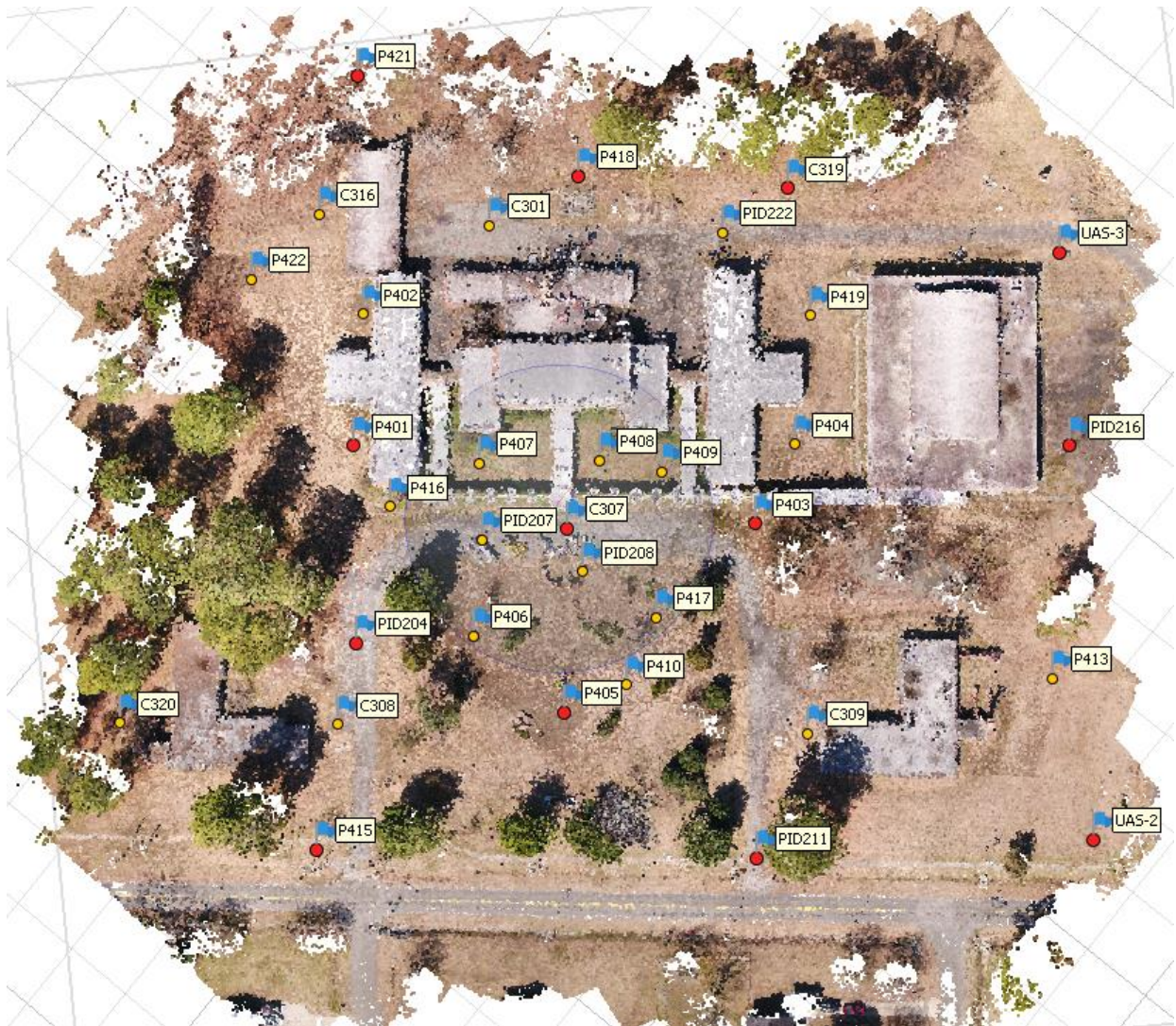
Figure 9.2 The Layout of GCPs and Checkpoints
